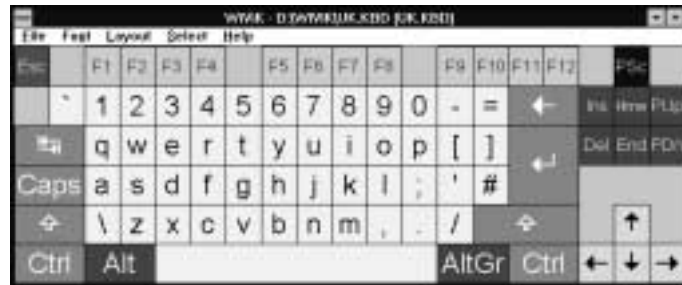
(b) WiVik on-screen keyboard accessed by single switch scan
